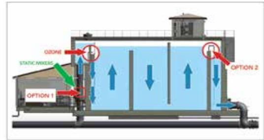
The system design includes two options for dosing hydrogen peroxide. In option 1, peroxide is fed prior to ozone addition to create hydroxyl radicals in AOP mode. In option 2, peroxide can be used at the end of the contactor to quench any ozone residuals.
