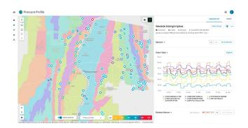
The Water Authority team simply logs onto a computer and opens the Pressure Profile application to view the latest data from smart meters and sensors on a map-based interface. Pressure zones, key assets and colored sensor icons offer a visual pulse of the system.
