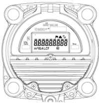
Segment Test View
