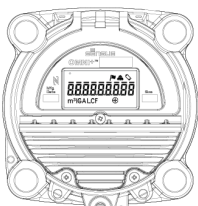
Segment Test View
